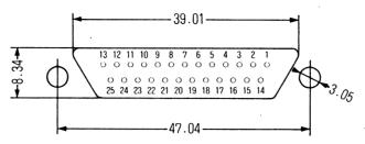
The size above is that of connector with cable. [units: mm]
