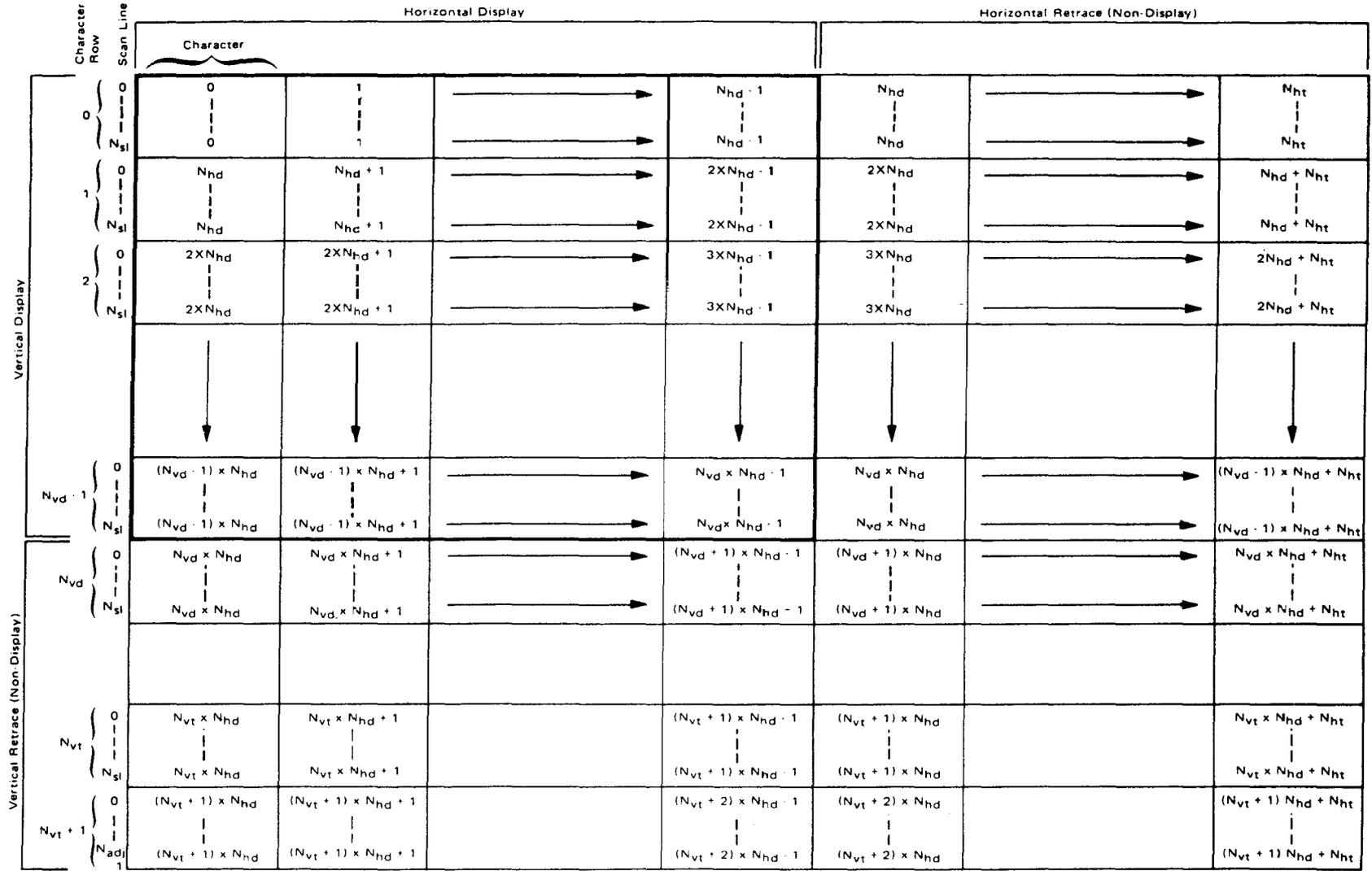
NOTE 1 The initial MA is determined by the contents of start address register, R12/R13. Timing is shown for R12/R13 = 0. Only Non-Interlace and Interlace Sync Modes are shown.
