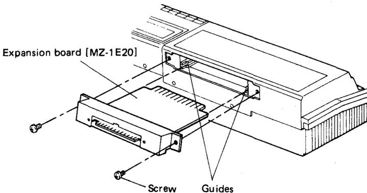
3. Connect the expansion unit connector to the expansion board and screw both ends of the connector.
