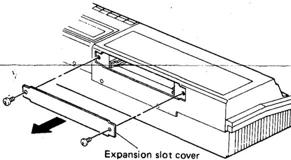
2. Insert the expansion board along the guides on both sides and firmly insert it into the connector mounted inside the slot. Affix it with the two screws to the rear panel of the MZ-800.
