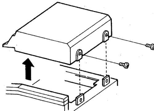
(3) Unplug the joint connector located inside the MZ-811.
