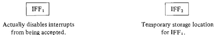
The state of IFF<sub>1</sub> is used to actually inhibit interrupts while IFF<sub>2</sub> is used as a temporary storage location for IFF<sub>1</sub>. The purpose of storing the IFF<sub>1</sub> will be subsequently explained.
